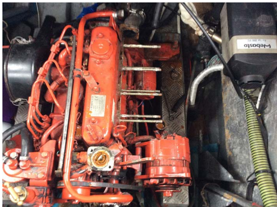
Cooling tank removed for repair and alternator lower right
